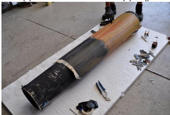
(d) Combustion chamber with upper half of fin can remaining.
